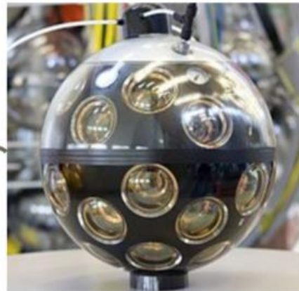
The KM3NeT DOM housing 31 3" PMTs
