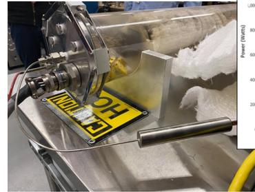
10-point TC installed and tested
