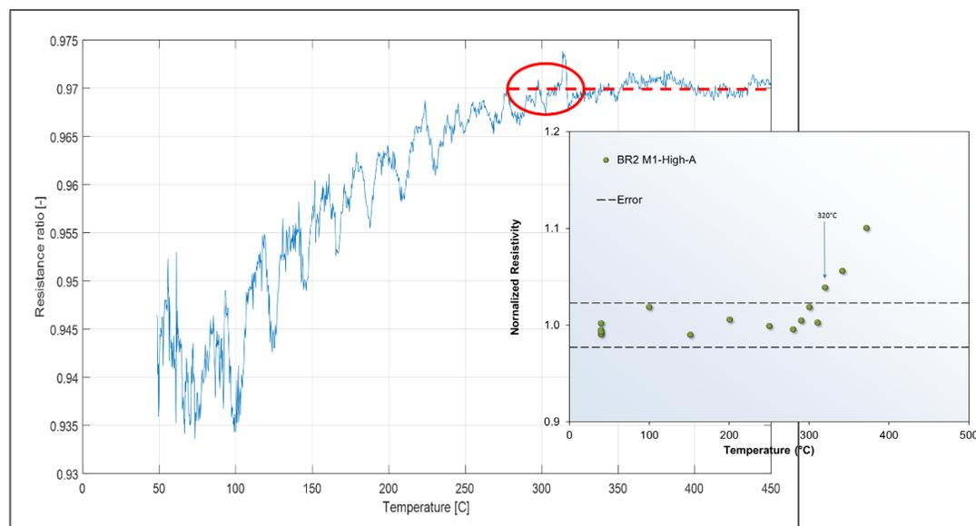
Continuous reading of SiC monitors in PIE after BR2 irradiation
