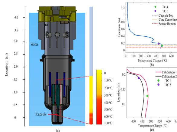
K. Chen (U Pitt) laser enhanced OFDR test in MITR and IFPI sensors fabrication
