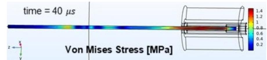
FEA model of 1.6 mm waveguide UT
