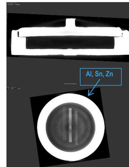
CT scan of printed Sn, Zn and Al melt wires
