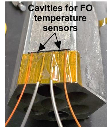
Core block with embedded sensors
