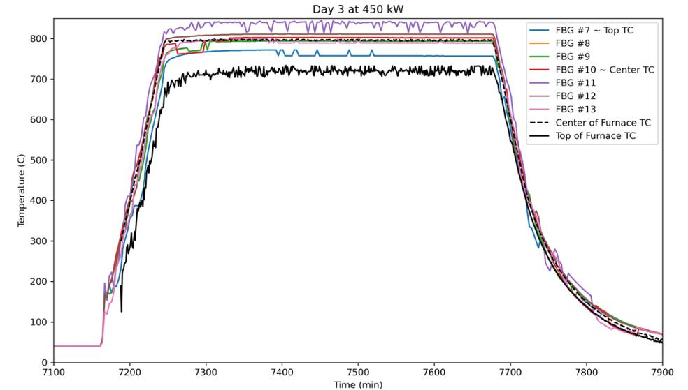
Sapphire optical fiber (75  $\mu\text{m}$  OD, clad via Li-6 method, with type-II FBGs) OFDR response at 800  $^{\circ}\text{C}$  and 450 kW reactor power (tested up to 1600  $^{\circ}\text{C}$ )
