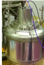
70 l detector sensitivity \sim 1-3 mBq/m 3
