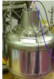
70 I detector sensitivity \sim 1-3 mBq/m 3
