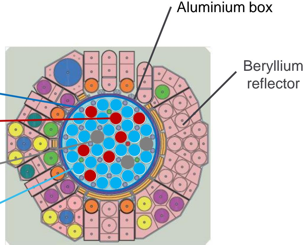
**20 simultaneous experiments (mobile or static devices) in core or reflector**
