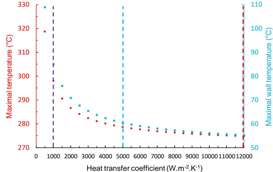
**When  $h$  increases from  $500\text{ W.m}^{-2}.\text{K}^{-1}$  to  $10000\text{ W.m}^{-2}.\text{K}^{-1}$ :**
