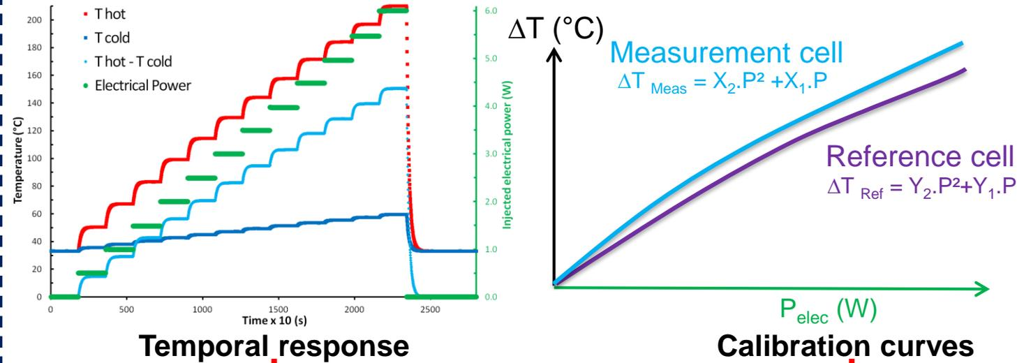
**Characterisation under laboratory conditions → response time, linearity and sensitivity**
