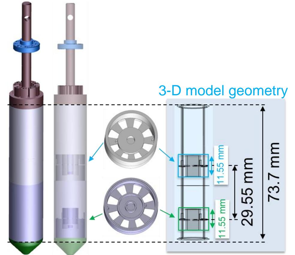
**New CALORRE cell design without spacers and heater holders and with a height equal to 73.7 mm**
