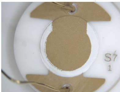
NBT devices with Au electrodes and Bounded Au wires
