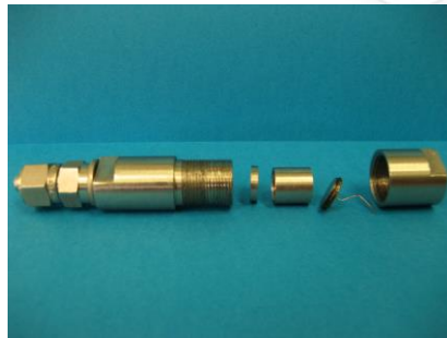
NDT sensor for measurement of gas composition [5]
