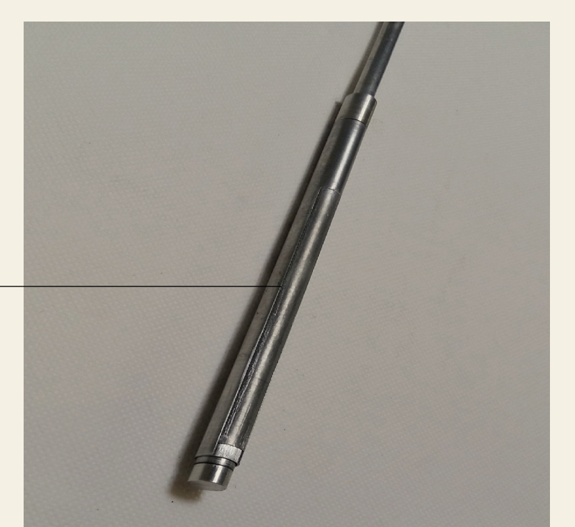
Rotor: 2 quarter circular cadmium strips of 100 mm length separated by 90° (0.46 g each), and an high density polyethylene bloc inside
