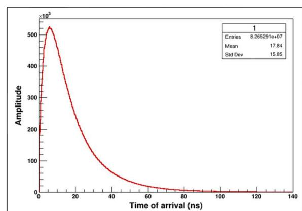
Figure 3. Average simulated pulse shape for EJ-276 scintillator in response to 2 MeV gamma rays
