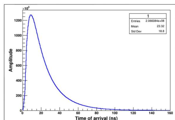
Figure 4. Average simulated pulse shape for EJ-276 scintillator in response to 2 MeV neutrons
