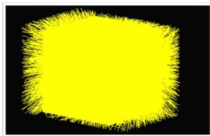
Figure 2. EJ-276 detector following interaction with > 1 gamma ray. Many scintillation photons are generated (shown in yellow)
