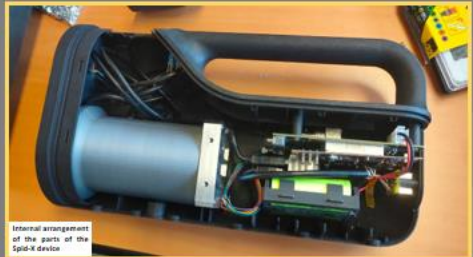
The device is 32.5 x 11 x 10 cm, for a weight under 3 kg
