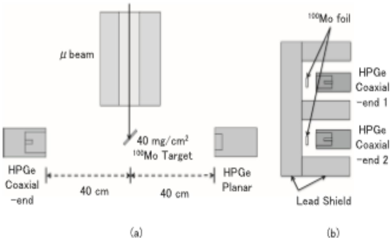
(a) Online setup for the  $\gamma$  rays with half-lived 0 to 1.5 hours.
