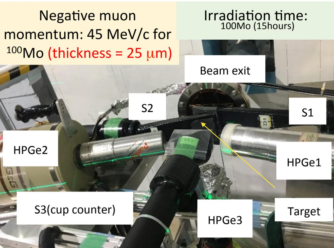
**3 trigger counters** with (S1•S2×S3)logic
